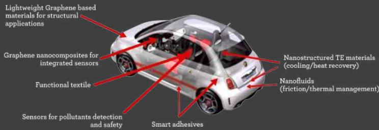
Figure 2. Graphene-based applications in a vehicle<sup>3</sup>
