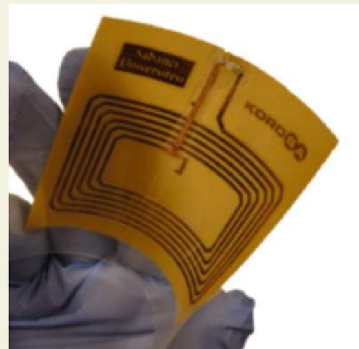
Figure 2: The first flexible sensor prototype developed by Sabancı University and Kordsa in April 2019.
