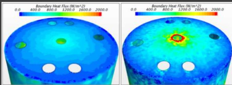
Figure 6: Heat flux distribution comparison of the top surfaces of the solidification chambers in Designs 1 & 2
