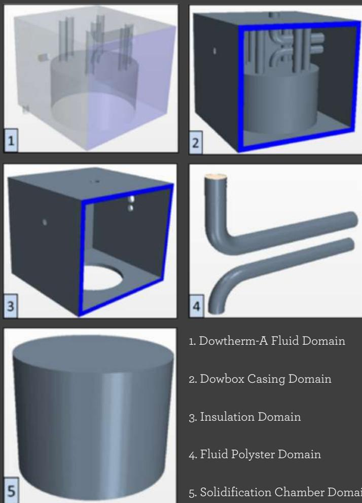
Figure 2: Heating box system model details
