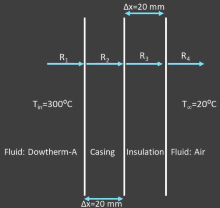
Figure 3: Resistances in the casing and insulation of the heating box system
