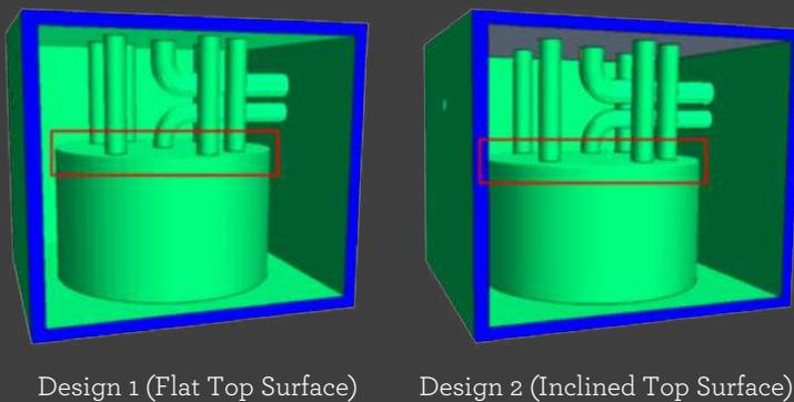
Fig 5: Fluid film thickness comparison for Design 1 & Design 2
