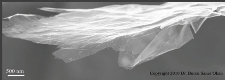
Figure 1. Electron microscopy image of graphene sheets
