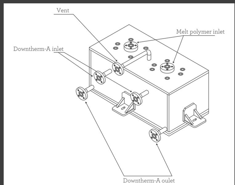
Figure 1: Schematic figure of a heating box (Dow-box)
